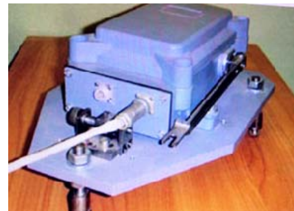
Fig. 2. The Stationary Structural Health Monitoring system.
